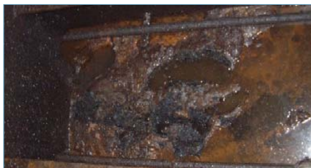
SLUDGE AND WATER REMAINING IN A VLCC'S TANK AFTER WATER WASHING
