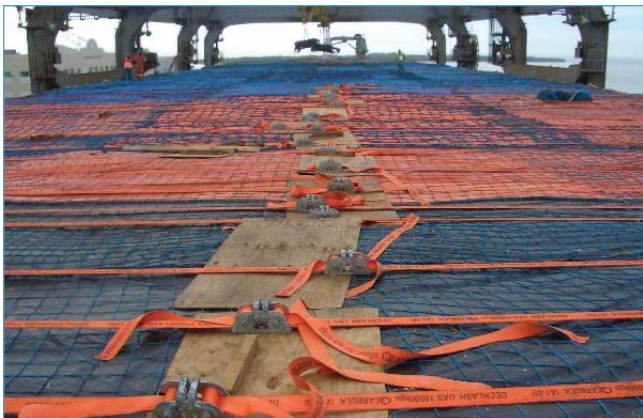
TIMBER DECK CARGO LASHINGS. PHOTO SUPPLIED BY CHECKMATE UK
