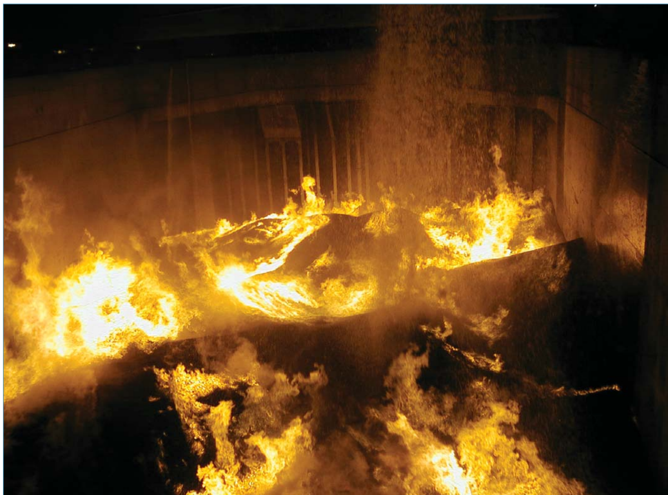
FIRE INVOLVING ‘PASSIVATED’ DRI PELLETS
