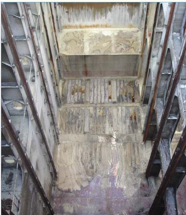
PHOTOGRAPH 1 – EXTENSIVE CONTAMINATION OF THE HOLD AFTER DECOMPOSITION OF THIOUREA DIOXIDE
