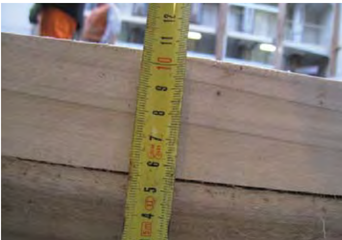
^Dunnage used should be adequate depth
