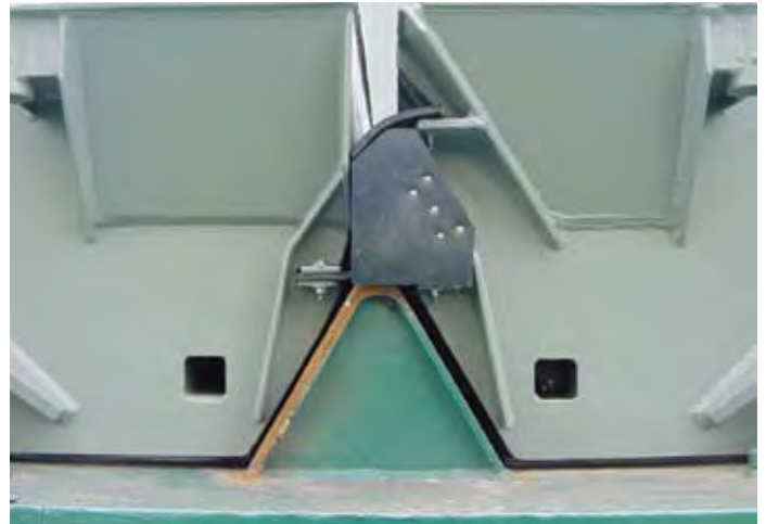
^ This sealing arrangement may be acceptable to Class; however, when subjected to an ultrasound test, it is likely to fail and therefore it is not recommended by the club for water-sensitive cargo. The only seal is a rubber seal/flap and a drain channel
