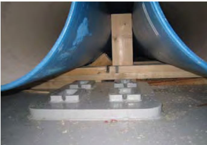
^ Dunnage keeping the cargo clear of tank top obstructions
