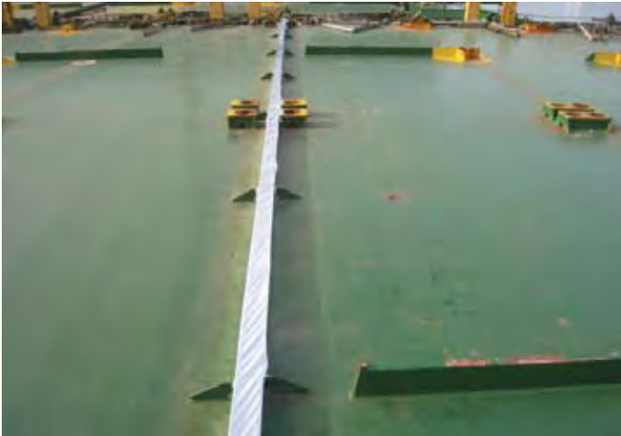
^ v The use of tape is not a primary means of preventing water ingress
