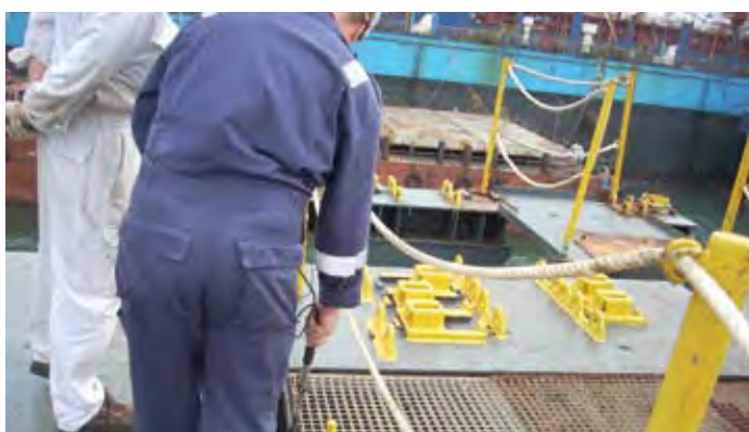
^Surveyors taking ultrasonic readings on hatch covers
