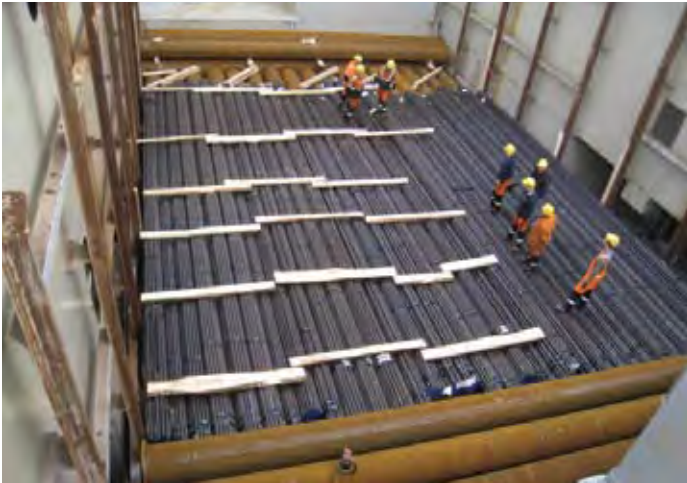
^Consider the tank top loading and stability. Tank top loading strengths should always be complied with
