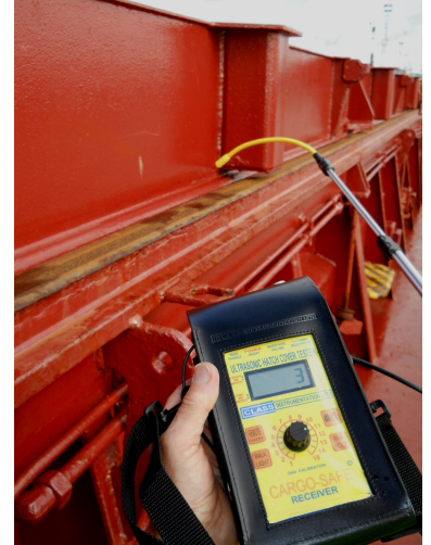
DNV surveyor checking hatch cover tightness.
