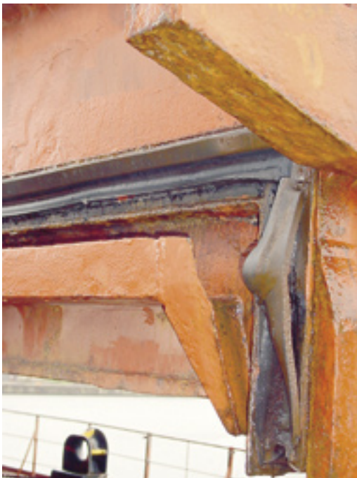
Attempt to upgrade seal with flat rubber.
