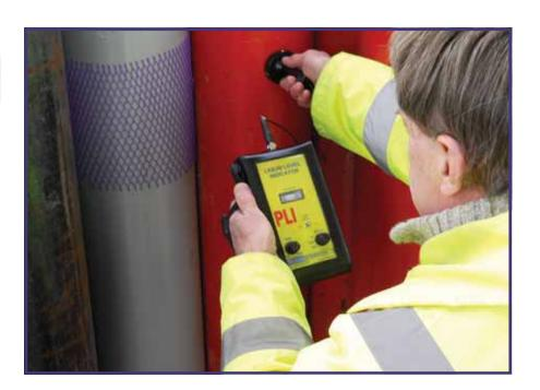
The PLI *Plus* Portable Liquid Level gauge is designed to offer a simple, accurate, rapid and reliable method of determining the liquid level of high or low pressure CO<sub>2</sub>, Halon, FM200, Propane and any liquefied gas under pressure, without the need to move or weigh the cylinders.
